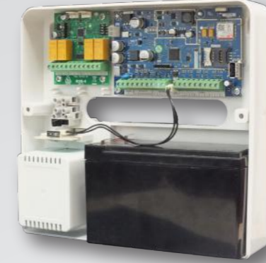
GPRS ALARM PANELİ
